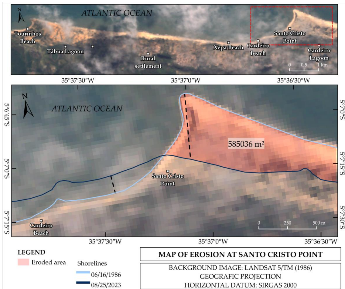
Figure 15. Eroded area at Santo Cristo Point between the years 1986 and 2023.
